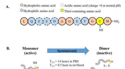
Fig. 1. A) Murine sequence of LR12 monomer peptide (Mr 1341 g/mol, calculated pl ~ 3.6) and B) main pathway of degradation by dimerization.
